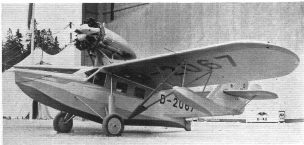
THE HEINKEL H.E. 57: In this three-quarter front view may be noticed the combined tail skid and water rudder. The airscrew tips pass very close to the windscreen and probably cause considerable buffeting. (FLIGHT Photo.)
